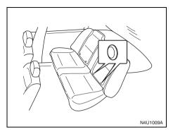
The disks are located near the base of the two rear outside seating positions.
